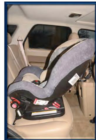
Car seat installed with lower anchor connectors
