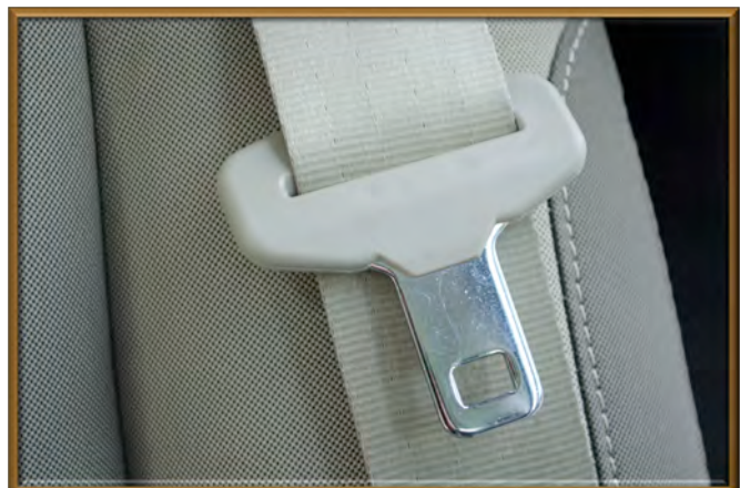
Sliding latchplate found only on lap-and-shoulder systems
