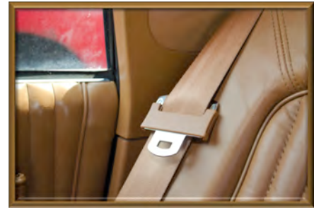
Locking latchplate with plastic piece
