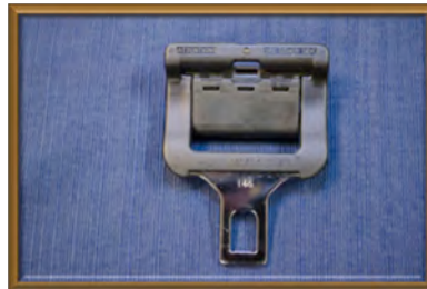
Locking parts from a switchable latchplate – front and back
