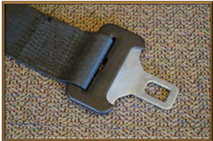
Sewn-on latchplate found on lap-only and lap-and-shoulder seat belts
