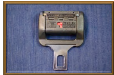
Locking parts from a switchable latchplate – front and back
